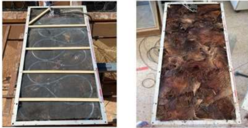
Figure II.2: Experimental setup of a photovoltaic cooling system using wet palm fibers in the Ouargla region [19]
