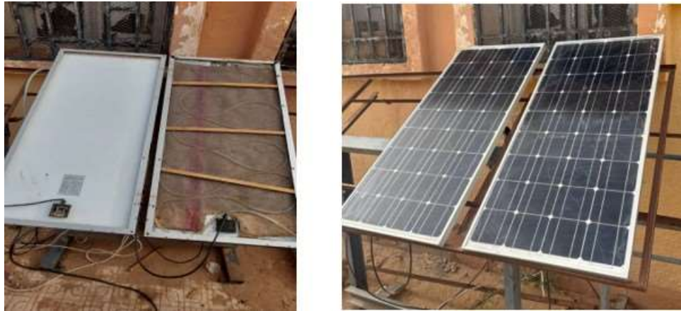
Figure III.5: Experimental Setup for Comparative Performance Evaluation between Cooled and Reference Panels
