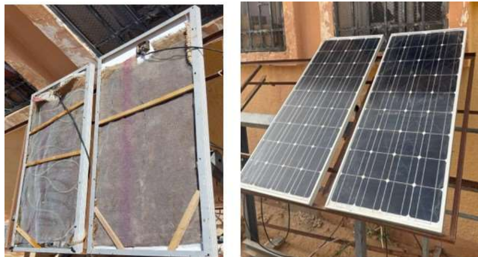
Figure III.6: Experimental Setup for Comparative Performance Evaluation between burlap cooling and hybrid burlap and newspaper cooling
