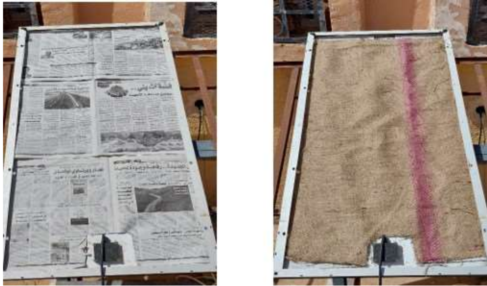
Figure III.1: Cooling Unit Components: Newspaper Layers and Jute Fibers
