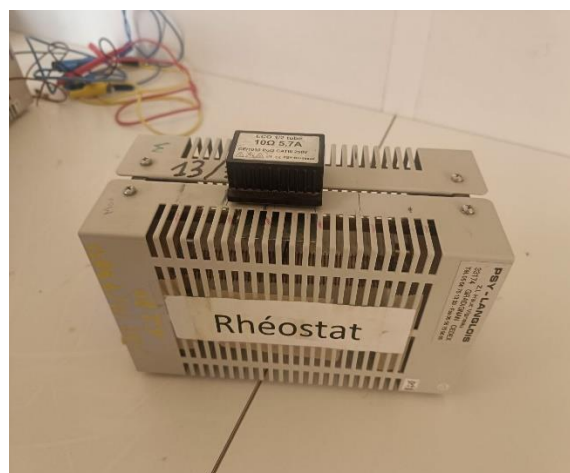
Figure III-8: ECO 1/2 tube-type power resistors.
