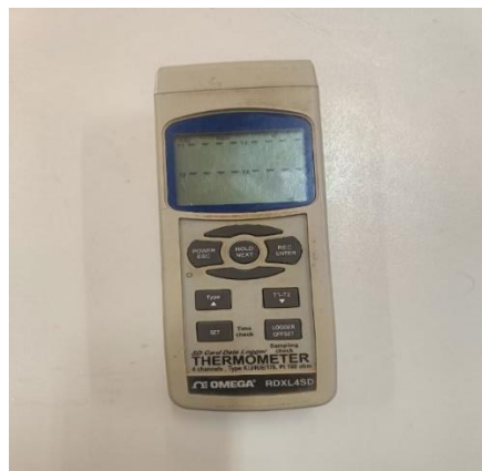
Figure III-6: OMEGA RDXL4SD four-channel digital thermometer.
