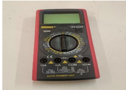
Figure III-7: DT-9205 digital multimeter.
