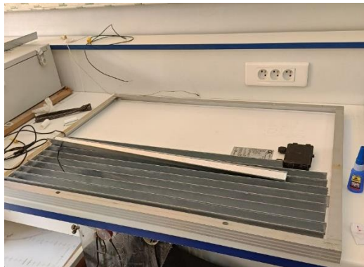
Figure III-11: Installation phase of the vertical galvanized steel fin array.
