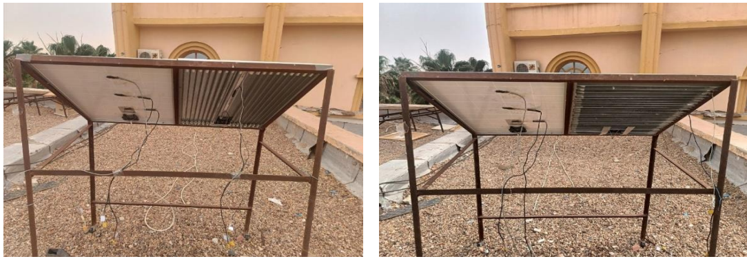
Figure III-13 : Completed vertical fin configuration field installation and Completed horizontal fin configuration field installation.
