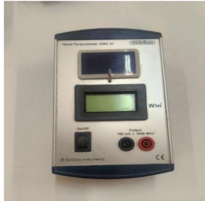
Figure III-9: Solar power sensor for solar irradiance measurement.
