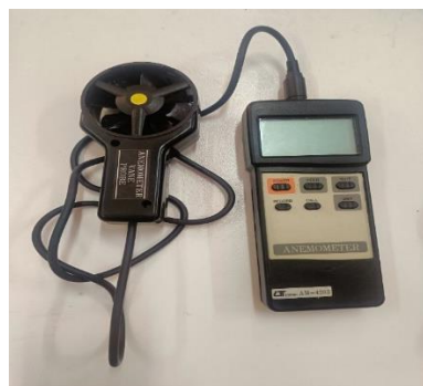
Figure III-10 : AM-4203 digital turbine anemometer.
