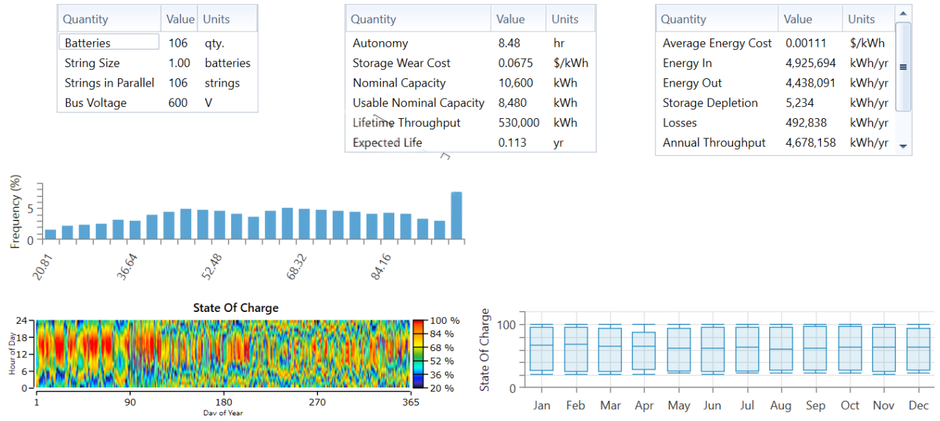
Figure 3-9 Scenario 2 HOMER configuration for the Storage system
