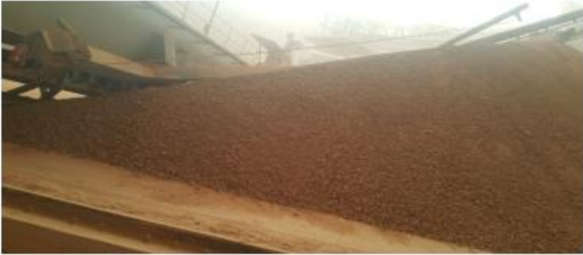
Figure 1-6 Pre-homogenization piling yard at the cement plant [2]
