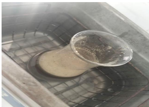
Figure 8 : Extraction mixture during ultrasonic-assisted extraction
