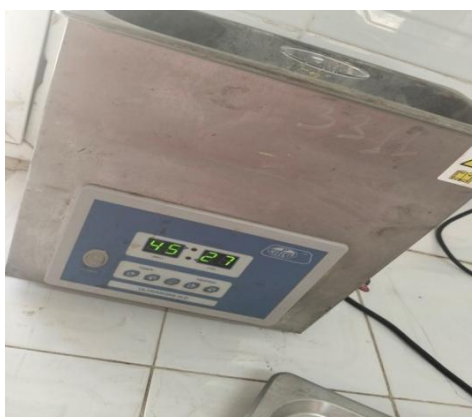
Figure 9 : Ultrasonic bath used for the extraction of bioactive compounds
