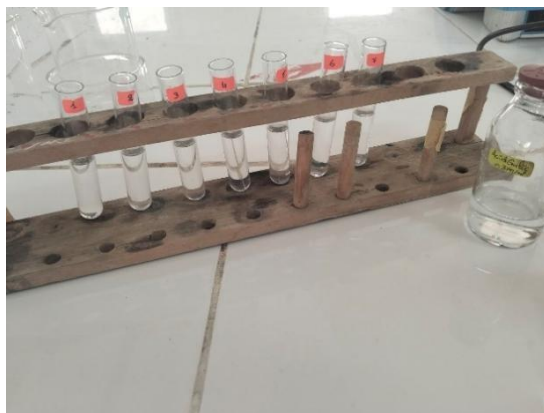
Figure 13 : Preparation of gallic acid standard solutions by serial dilution
