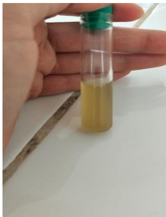
Figure 29 : (B) Fading of the yellow color after addition of dilute \text{HCl}
