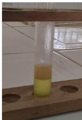
Figure 35 : Qualitative detection of terpenoids in Anabasis articulata extract by the Salkowski test
