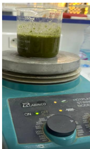
Figure II-22: Mixing Neem powder in a magnetic stirrer
