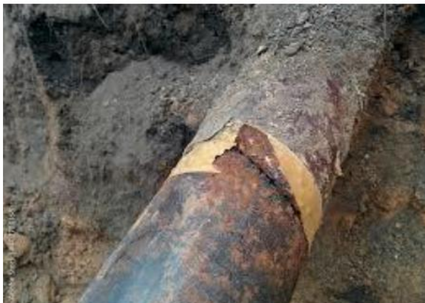
Figure III-3 :Perforation Level of 4" pipe
