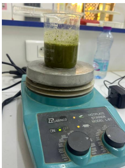
Figure II-15: Mixing Oregano powder in a magnetic stirrer
