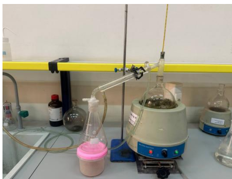
Figure II-10 : Rosemary oil extraction process
