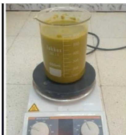
Figure II-8 : Mixing rosemary powder in a magnetic stirrer
