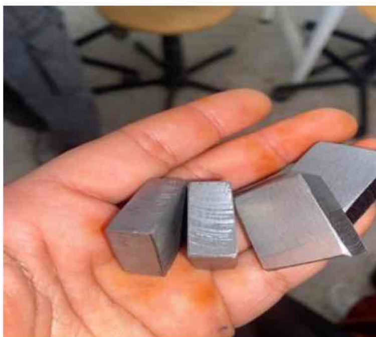
Figure III-6: the steel sample after polishing
