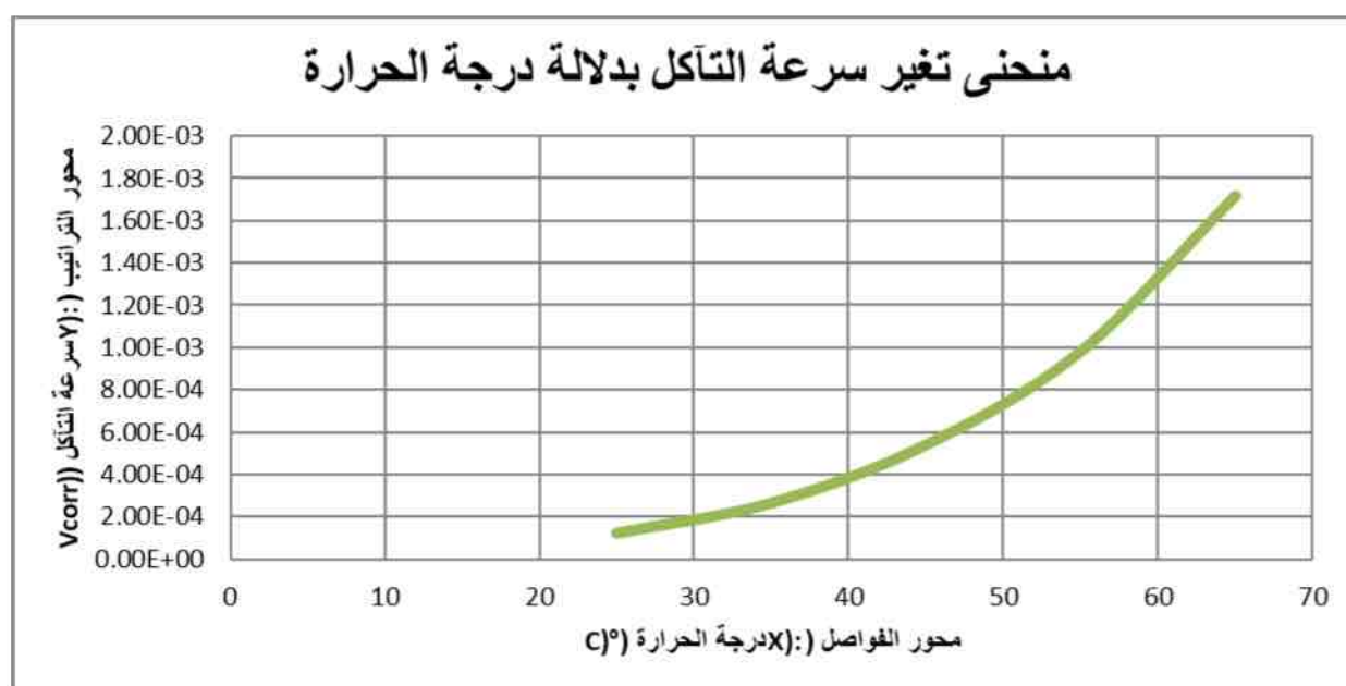
Figure III.10: Corrosion Rate as a Function of Temperature
