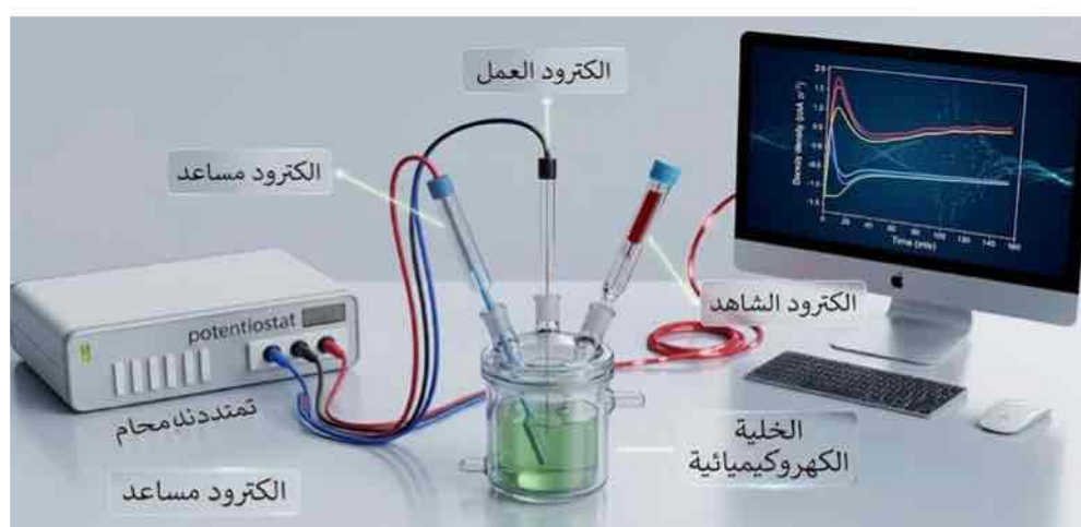
Figure III-16: Schematic diagram of the electrochemical cell setup
