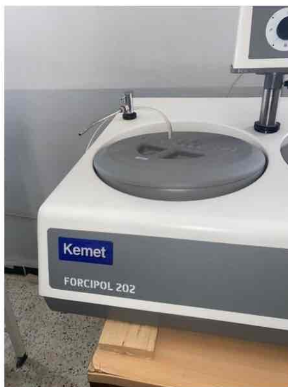
Figure III-1: Mechanical polishing device
