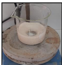
Constant stirring of the mixture of TiO 2 and Chard leaf extract.
