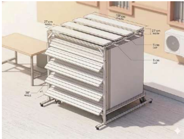
Figure 2-7 AI-assisted 3D render of the test cell setup showing the specifications of the external shading system.
