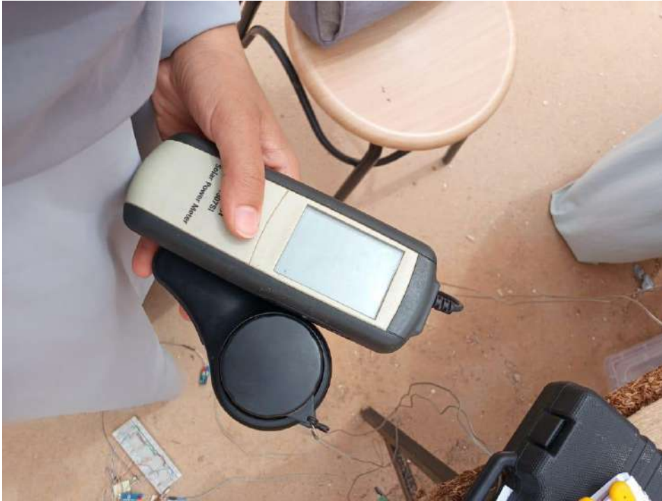
Figure 2-10 The experimental Solar Radiation device (Pyranometers)
