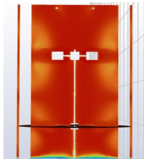
Figure 4-4 volume fraction of sand on YZ view
