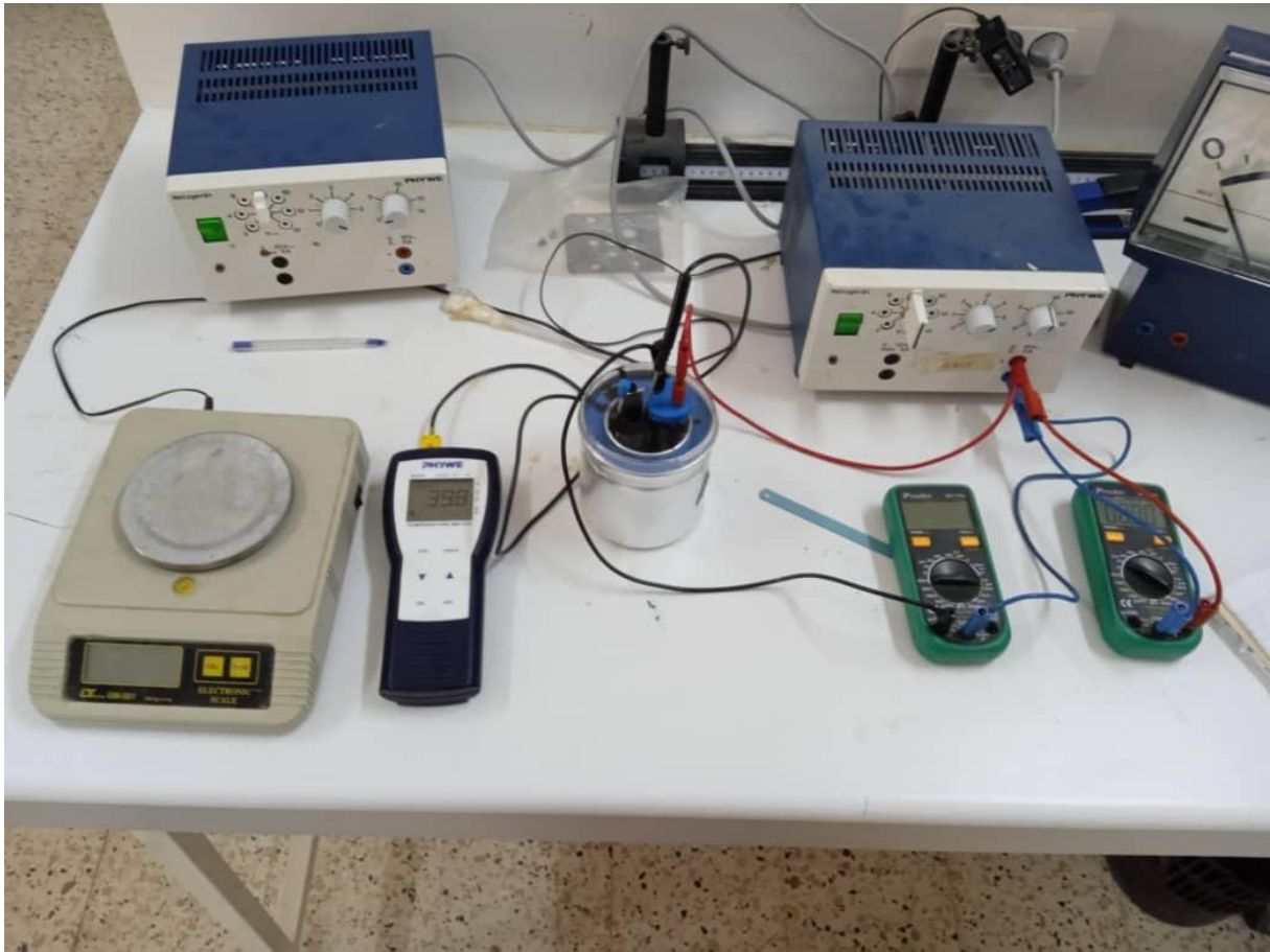
Figure III.5.1.2 Laboratory apparatus and electrical circuit used for oil specific heat capacity ( C_p ) determination.
