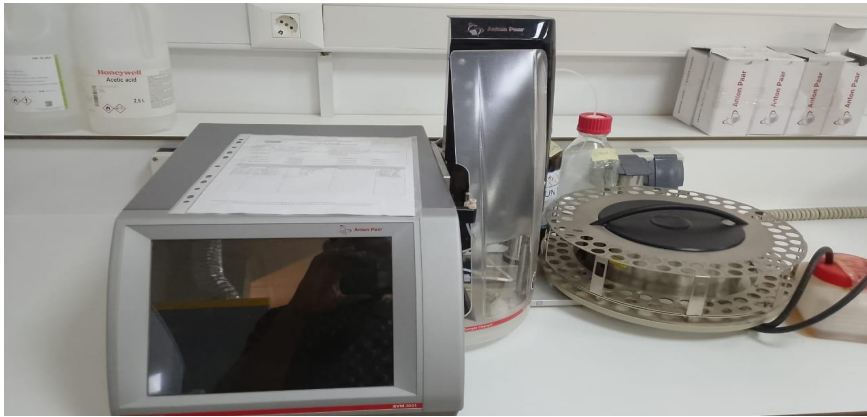
Figure III.5.1.1 Laboratory apparatus used for measuring HTF kinematic viscosity and density
