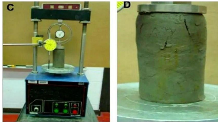
Figure I-5 unconfined compressive strength test
