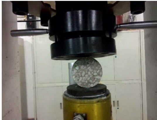
Figure I-6 Brazilian tensile strength test
