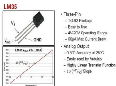
Figure 3-12: LM35 temperature sensor for overtemperature protection.
