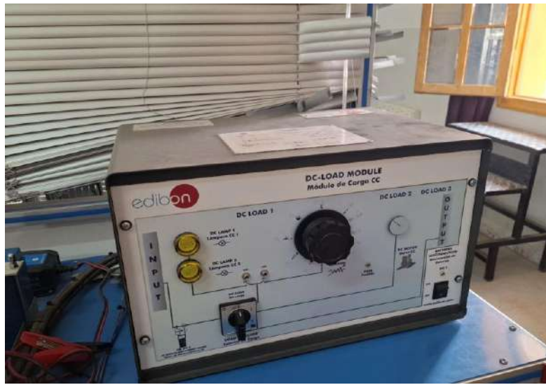
Figure 2.7: DC Load Module.
