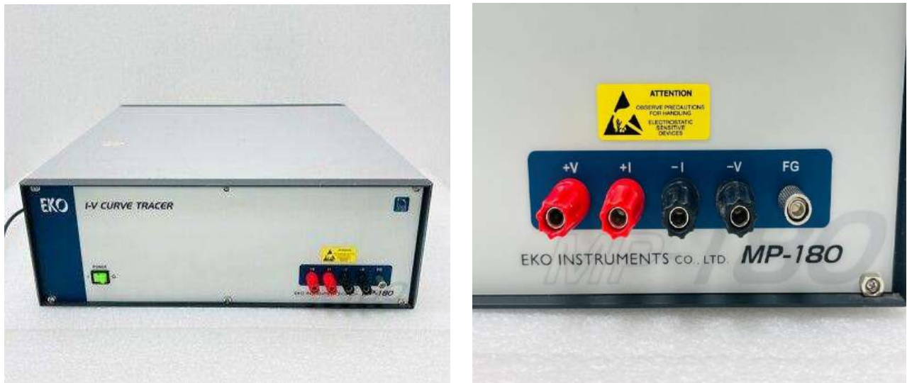
Figure 2.4. EKO Instruments MP-180 high-precision laboratory benchtop I-V tracer for PV cell research.
