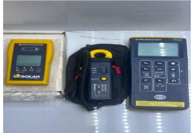
Figure 2.3. Seaward PV200 compact handheld I-V curve tracer with wireless irradiance meter (Source: Seaward Electronic Ltd.).
