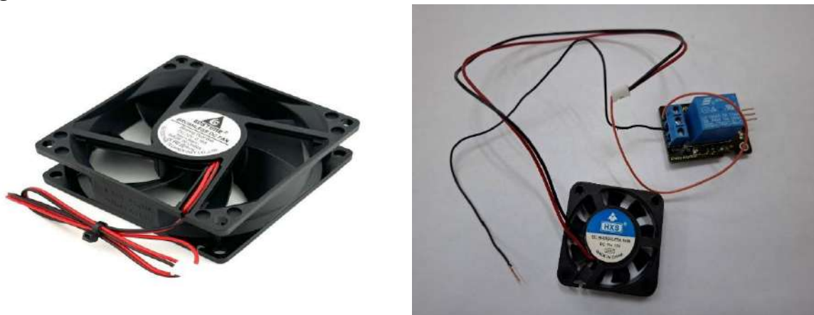
Figure 3-8: 12V DC cooling fan for MOSFET active thermal management.
