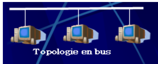
Figure 1.2: Topologie en bus.
