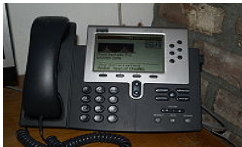
Figure 3.19: Terminal SIP CISCO 7960G
