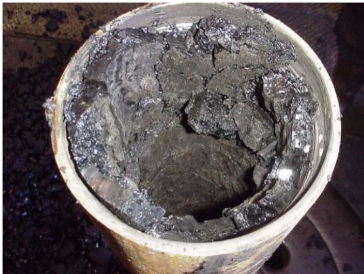
Figure. II.4. déposition Asphaltènes (source: 2007Petroskills LLC. All Rights Reserved)
