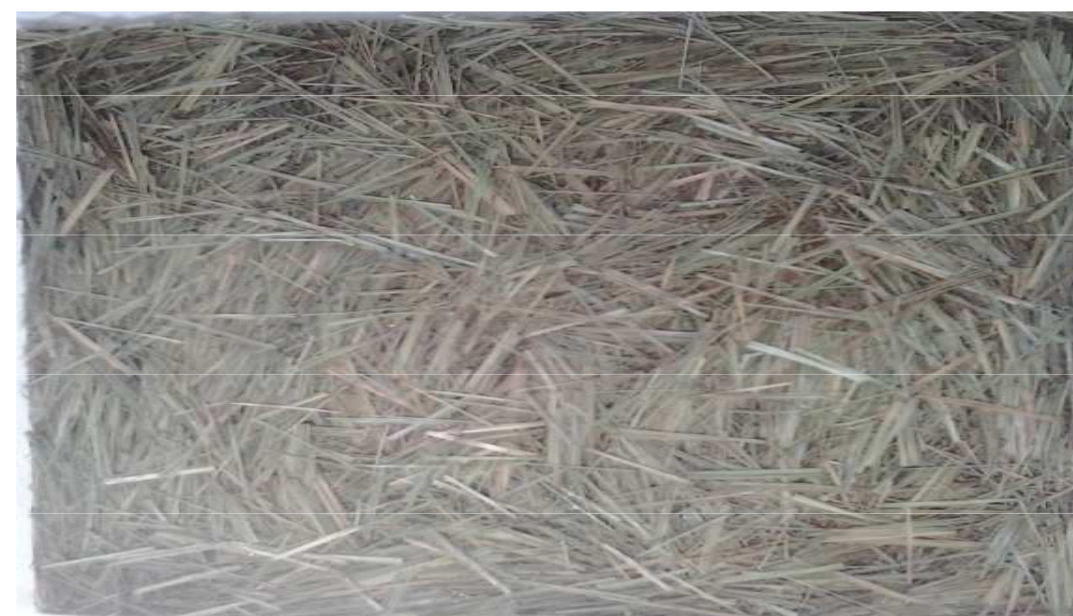
Fig.5 : plaque composite obtenue (diss / polyester)
