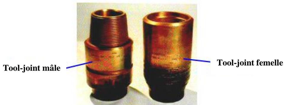
Figure N° II-05 : Tools- joints
