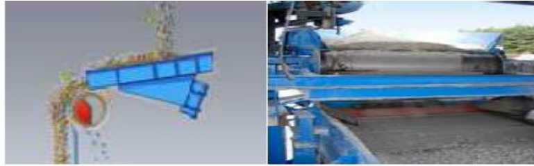
Figure I.21: Tambour à aimant permanent
