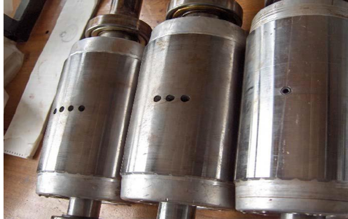
Fig I-5 Rupture de barre
