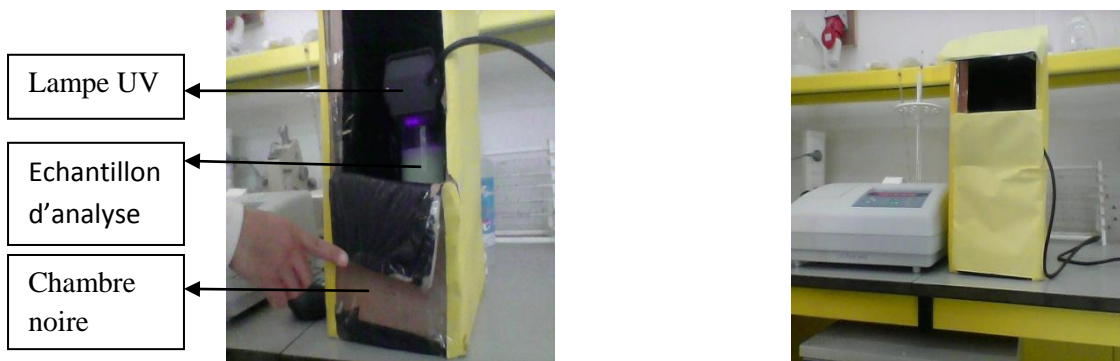
Figure (5) : montage photocatalyse TiO 2 /UV
